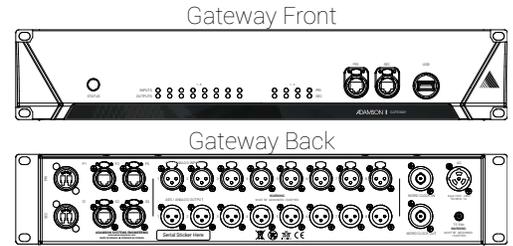
**Bridge (913-0005)** - The Bridge is designed to replace existing network infrastructure in Adamson's E-Rack, allowing users to seamlessly integrate CS-Series loudspeakers into their existing inventories by converting dual-LAN, Milan AVB signal to AES/EBU for networking to existing Lab Gruppen amplifiers, while also offering six channels of DSP per unit.
