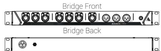
**Network Distribution System NDS (905-0039)** - The NDS is a network and analog patch bay that allows users to send redundant audio and control to CS-Series loudspeakers on a single network cable. The NDS combines LAN A and B network ports using two external AVB enabled switches.
