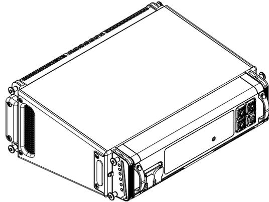
The CS7 is an ultra-compact, powered, intelligent, line array enclosure designed for medium throw applications. It contains two symmetrically arrayed 7" LF transducers, and a 3" HF compression driver mounted onto an Adamson waveguide. The high frequency waveguide is designed to couple multiple cabinets across the entire intended frequency band without loss of coherence.
